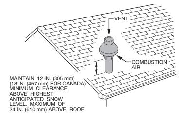
Fig. 40—Concentric Vent and Combustion-Air RoofTermination (Preferred)
